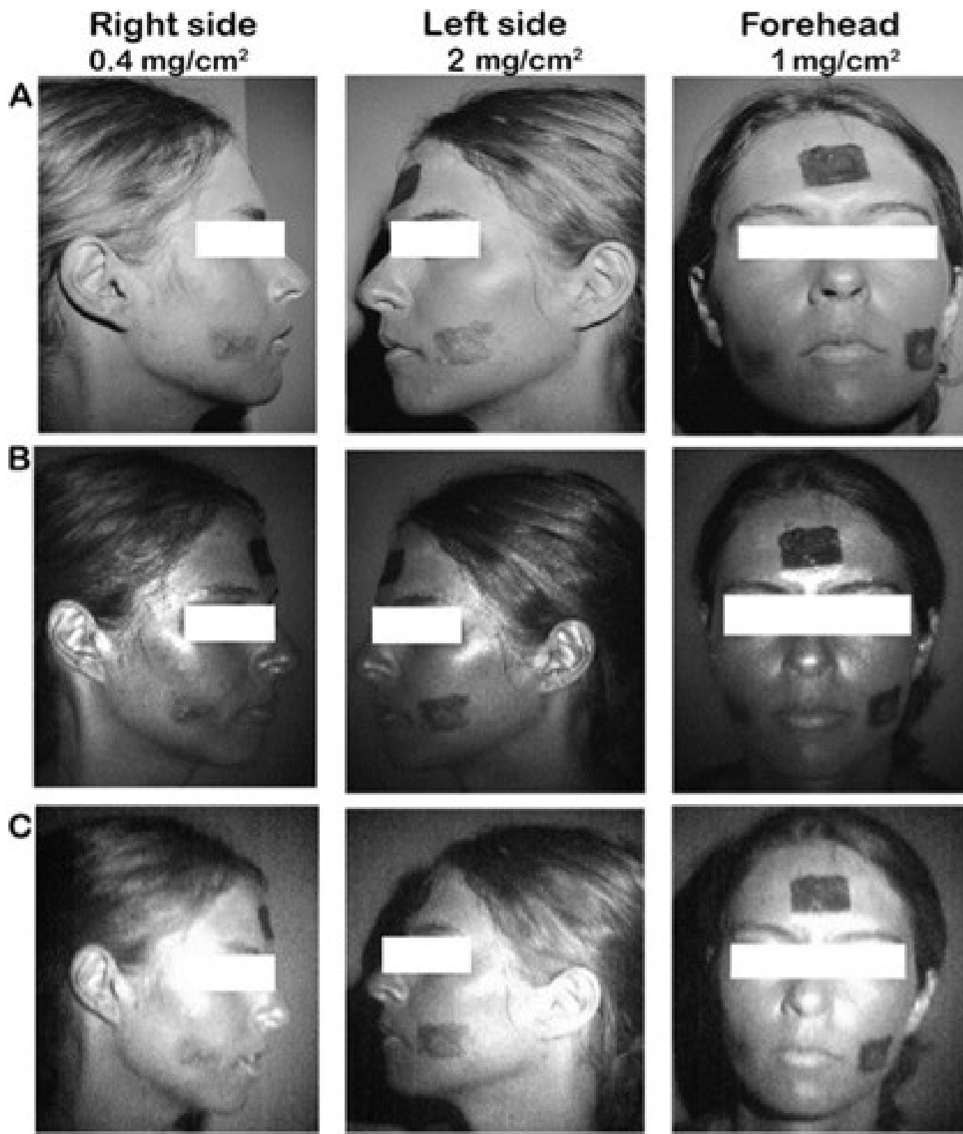
Figure 2-2. Comparison of UV Photography Device Images of Sun Protection Factor (SPF) 50+ Lotion Applied to a 4 \times 2.5\text{-cm}^2 Area of the Cheeks and Forehead: (A) DSLR UV Camera, (B) Nurugo SPF Camera, and (C) Sunscreen Camera (Source: Horsham et al. [79]).
